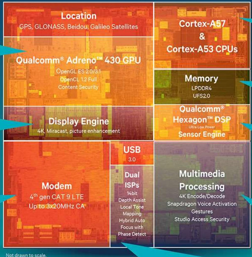
Qualcomm Technologies' FIRST 14-bit Dual ISP for highest quality, depth enabled photography. Up to 21MP for main camera with depth assist, phase detect, for sharper dual camera user experiences
